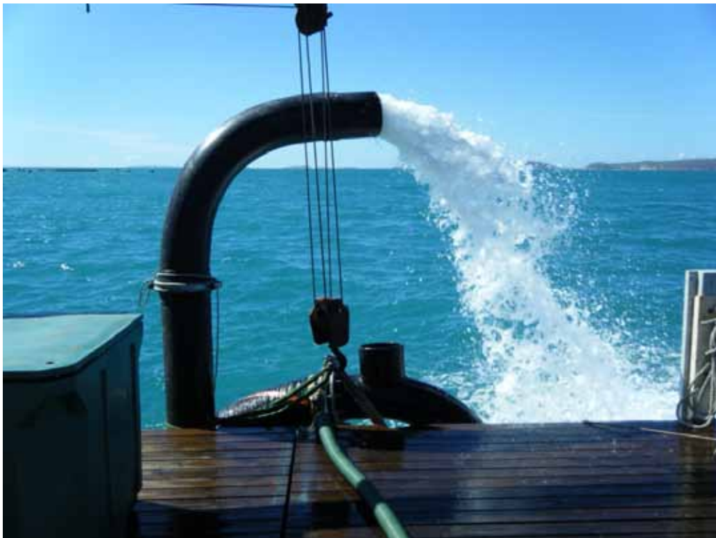
Airlift pump during testing. Unobstructed flow gentle on fish during pumping
